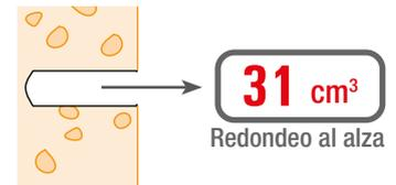
$$\text{VOLUMEN (cm}^3\text{)}_{\text{VARILLA}} = \frac{3.1416 \times 1.2 \times 1.2 \times 20}{4} = 22.62 \text{ cm}^3$$
